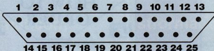
Looking into the 25 - Pin D plug (printer plug)
